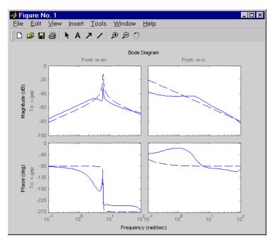
The dashed lines show the open-loop response. Note that the peak gain of the eccentricity-to-gap response and the low-frequency gain of the input-thickness-to-gap response have been reduced by about 20 dB.
