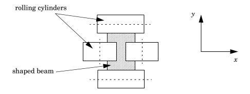
This shape is impressed by two pairs of rolling cylinders (one per axis) positioned by hydraulic actuators. The gap between the two cylinders is called the *roll gap*.
