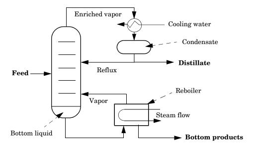
Figure 1-3: Distillation Column
