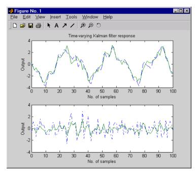
The first plot shows the true response y (dashed line) and the filtered response  $y_e$  (solid line). The second plot compares the measurement error (dash-dot) with the estimation error (solid).
