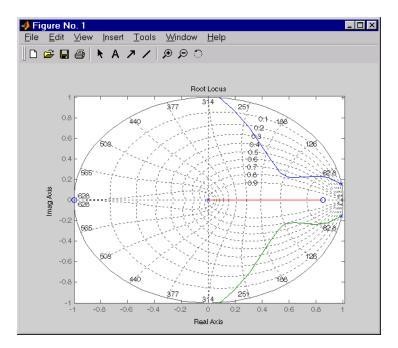
This time, the poles stay within the unit circle for some time (the lines drawn by zgrid show the damping ratios from  $\zeta=0$  to 1 in steps of 0.1). Use a data
