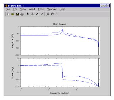
The plot above shows that the compensator has shifted up the phase plot (added lead) in the frequency range  $\omega > 10 \, \text{rad/sec}$ .
