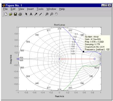
marker to find the point on the curve where the gain equals 4.111e+03. This figure shows the data marker at the correct location.
