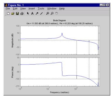
This design is robust and can tolerate a 11 dB gain increase or a 40 degree phase lag in the open-loop system without going unstable. By continuing this design process, you may be able to find a compensator that stabilizes the open-loop system and allows you to reduce the seek time.
