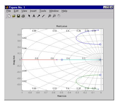
This looks better. By using simple feedback, you can achieve a damping ratio of  $\zeta=0.45$ . Click on the blue curve and move the data marker to track the
