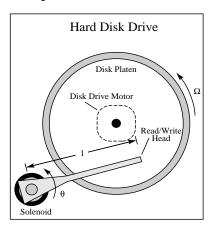
This case study demonstrates the ability to perform classical digital control design by going through the design of a computer hard-disk read/write head position controller.
