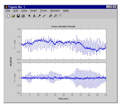
The response reveals a severe deterioration in regulation performance along the *x*-axis (the peak thickness variation is about four times larger than in the simulation without cross-coupling). Hence, designing for one loop at a time is inadequate for this level of cross-coupling, and you must perform a joint-axis MIMO design to correctly handle coupling effects.
