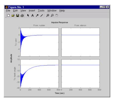
The impulse response confirms that the system is lightly damped. But the time frame is much too long because the passengers and the pilot are more concerned about the behavior during the first few seconds rather than the first few minutes. Next look at the response over a smaller time frame of 20 seconds.
