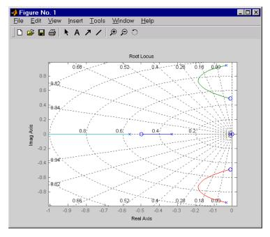
Create and drag a data marker around the upper curve to locate the maximum damping, which is about  $\zeta=0.3$ .
