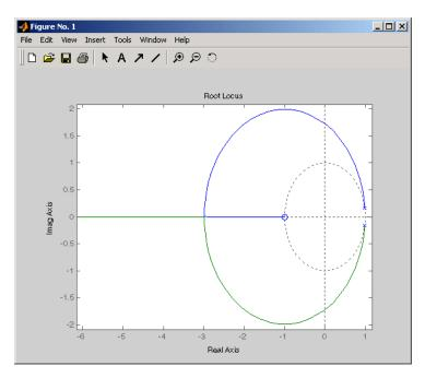
As shown in the root locus, the poles quickly leave the unit circle and go unstable. You need to introduce some lead or a compensator with some zeros.
