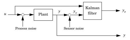
You can construct a state-space model of this block diagram with the functions parallel and feedback. First build a complete plant model with u, w, v as inputs and y and  $y_v$  (measurements) as outputs.
