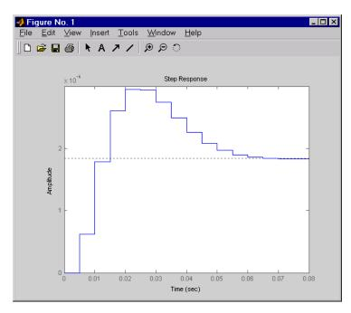
This response depends on your closed loop set point. The one shown here is relatively fast and settles in about 0.07 seconds. Therefore, this closed loop disk drive system has a seek time of about 0.07 seconds. This is slow by today's standards, but you also started with a very lightly damped system.
