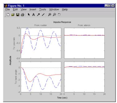
The bank angle response (output 2) due to an aileron impulse (input 2) now has the desired nearly constant behavior over this short time frame. To inspect the
