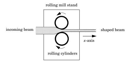
The objective is to maintain the beam thickness along the *x*- and *y*-axes within the quality assurance tolerances. Variations in output thickness can arise from the following:
